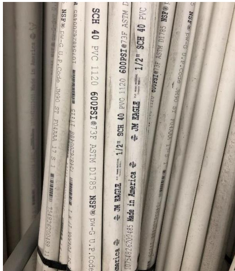
Potable white PVC line with NSF label PVC pipe
