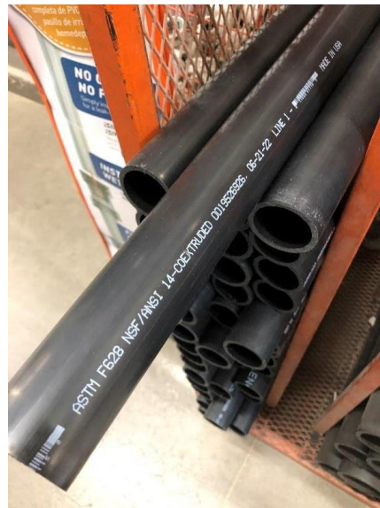
Non-potable/wastewater black PVC pipe
