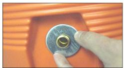
Place round metal washer over nipple on the outside of water cooler
