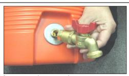
Screw-in close nipple to pipe bushing
